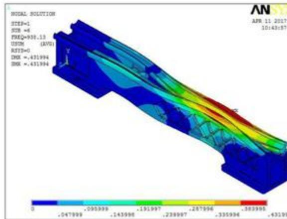
Fig 23: Natural Frequency mode – 6 Deformation
