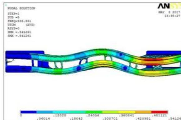
Fig 32: Natural Frequency mode – 5 Deformation
