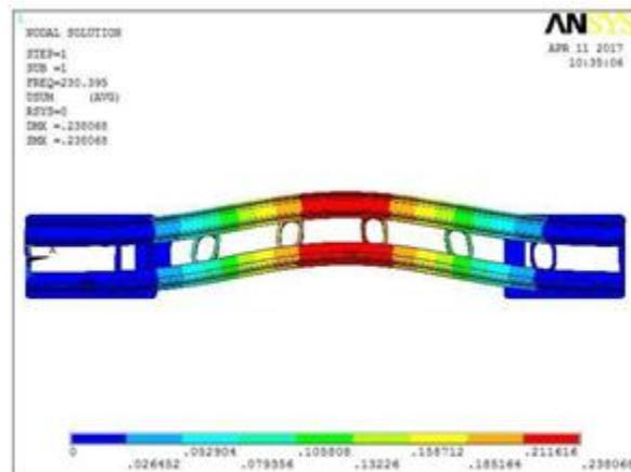
Fig 18: Natural Frequency mode – 1 Deformation
