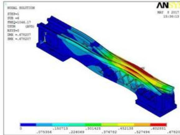
Fig 33: Natural Frequency mode – 6 Deformation
