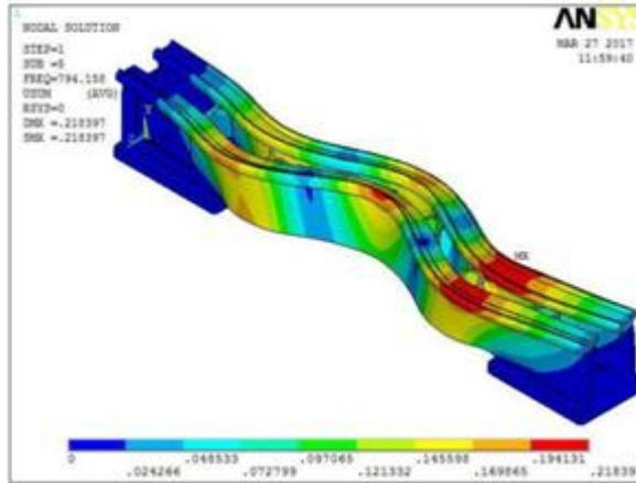
Fig 12: Natural Frequency mode – 5 Deformation
