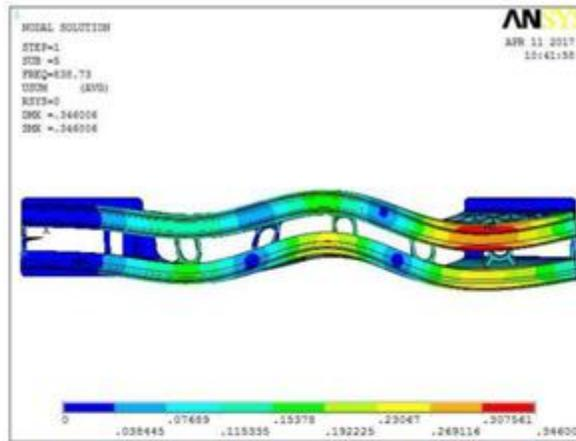
Fig 22: Natural Frequency mode – 5 Deformation
