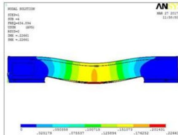
Fig 11: Natural Frequency mode – 4 Deformation
