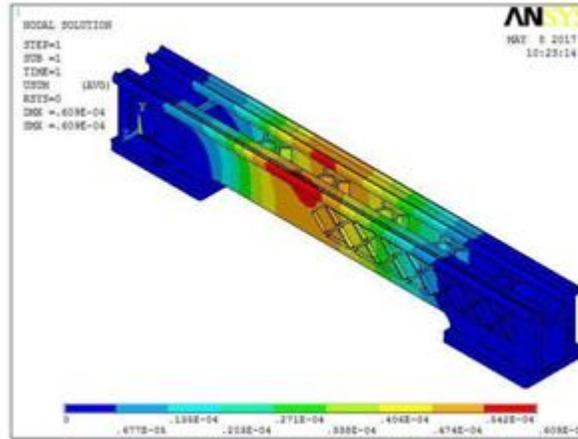
Fig 25: Deformation of lathe bed before weight optimization
