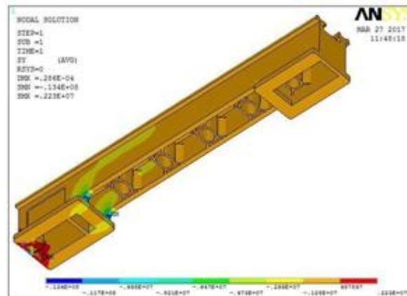
Fig 6: Stress Distribution of lathe bed in Y direction before modification
