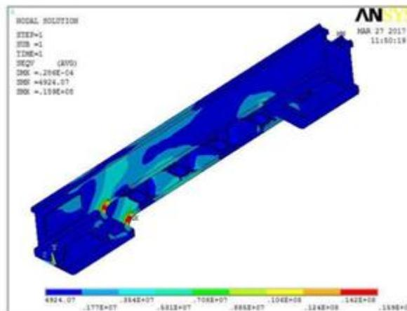
Fig 7: Von-mises stress Distribution of lathe bed before modification
