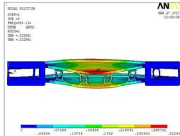
Fig 10: Natural Frequency mode – 3 Deformation
