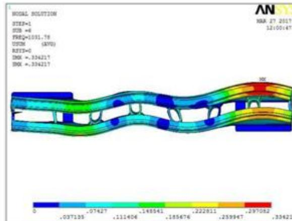
Fig 13: Natural Frequency mode – 6 Deformation
