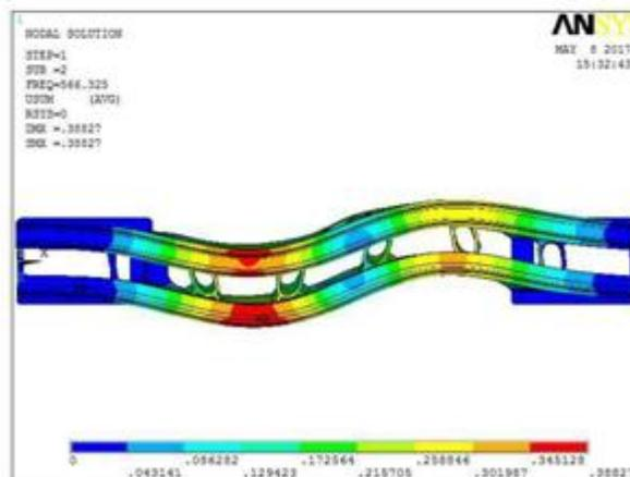
Fig 29: Natural Frequency mode – 2 Deformation
