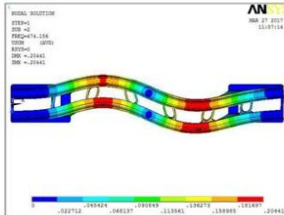
Fig 9: Natural Frequency mode – 2 Deformation
